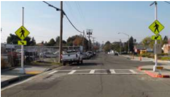
46. View of crosswalk from the driver's perspective (one way, single lane road)
