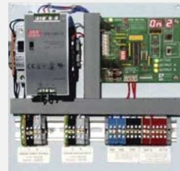
Color coded terminal blocks reduce installation time.
